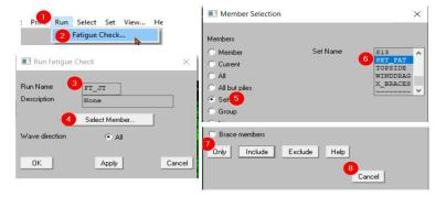
After the analysis completed, go to Print > Fatigue Check Results, select the analysis results to be printed into the listing file for tubular connections included in set SET\_FAT.
