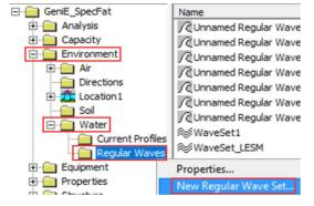
In the dialog box, name this new wave set as WaveSet\_Dynamic and add at least 96 (total number of seastates) lines by using \u221d downward key on the keyboard.
