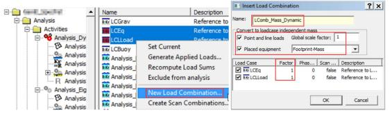
Since a Splice analysis will be performed after the dynamic analysis, a load combination containing all vertical loads, such as the structural self-weight, equipment loads, deck live loads, marine growth weight, and all buoyancies, need to be created. The calculated dynamic effect plus the loads in this load combination will be included in the static Splice analysis.
