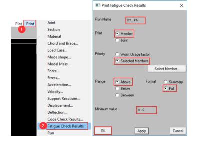
The fatigue analysis results for pile butt-welds are listed in the file located in **Framework\_SpecFat** activity folder.
