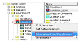
Define the wave condition name as Condition\_Dynamic, select wave set WaveSet\_Dynamic, use Airy as wave model for all waves, and then include two additional seastates with CalmSea wave model.
