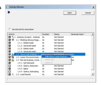
• Edit the wave load activity in the newly created analysis. Set the wave step length to 12 degrees, the number of steps to 31. Set buoyancy calculation **Off** and doppler effect **Off**, then click **Fill all**. Click **Apply** to save the input but keep the dialog box open.
