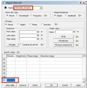
Copy wave Period, Height, Phase angel, and Direction for all waves from the Excel spreadsheet and then paste them into this wave set.
