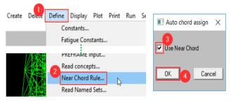
**NOTE:** This will ensure that the chord member and the aligned chord member of a brace do not change when the structure and its load pattern are subject to a rotation. This is useful when multiple fatigue analyses are performed on the same model in different states, e.g. when the model is standing and when the same model is placed horizontally for transportation in another fatigue analysis. This ensures that the hotspots are the same in both analyses, so that results can be summed correctly.
