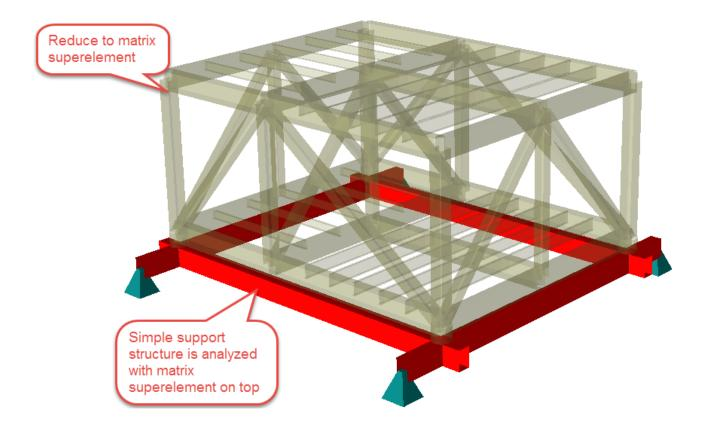
This document explains the example ExportImportMatrixSuperelement. The example shows how to create a matrix superelement by reducing a standard superelement created in GeniE. The advantages of using a matrix superelement compared to using the standard superelement on which it is based are:
