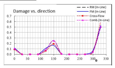
The "Damage distribution vs. direction" chart shows the normalized contribution each direction relative to geographic North has to the individual fatigue components, i.e., in-line response model, in-line force model, combined in-line fatigue life and cross-flow fatigue life.
