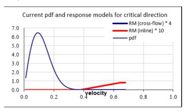
The pdf graph indicates the likelihood of cross-flow or in-line motion occurring from the critical direction current flow alone. The effect of waves can be evaluated by adding the wave induced flow velocities to the long-term current probability density function in the figure. Safety factors are included.
