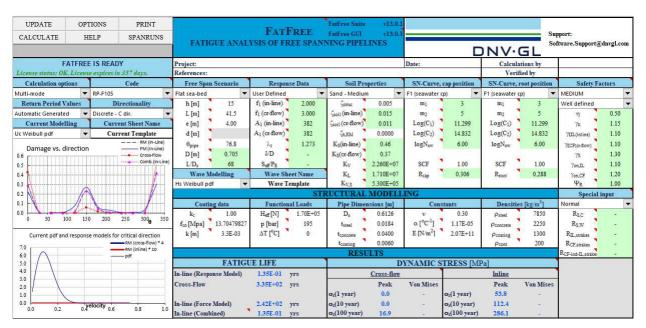
The program has been designed so that the majority of the input and results are located on the "MAIN" sheet, i.e., the user can see all the necessary information from this sheet without navigating between many windows.
