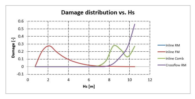
The "Damage distribution" chart shows the contribution each significant wave height (averaged over the wave periods) has to the individual fatigue components, i.e., in-line response model, in-line force model, combined in-line fatigue life and cross-flow fatigue life.
