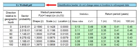
Here, the three Weibull parameters are given together with the sector probability of occurrence for different directions. Dimensionful parameters,  $\alpha$  and  $\gamma$ , are defined in [m/s].
